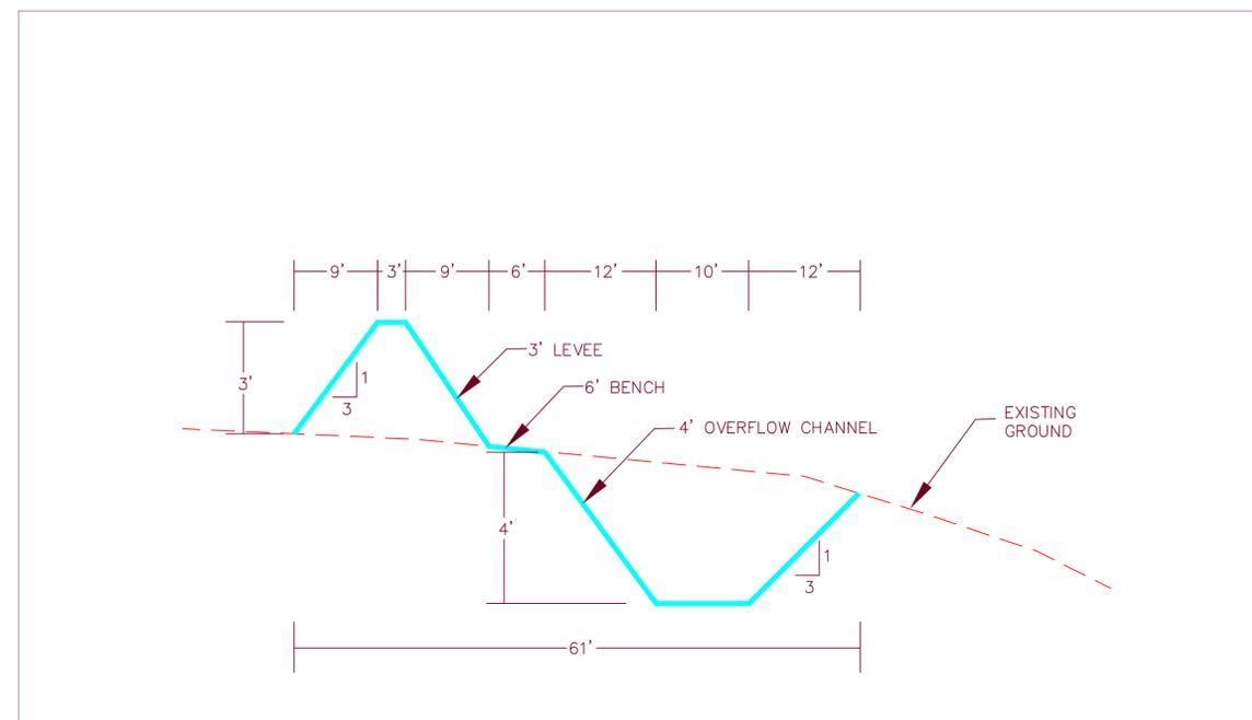
**LEVEE AND OVERFLOW CHANNEL DETAIL**
