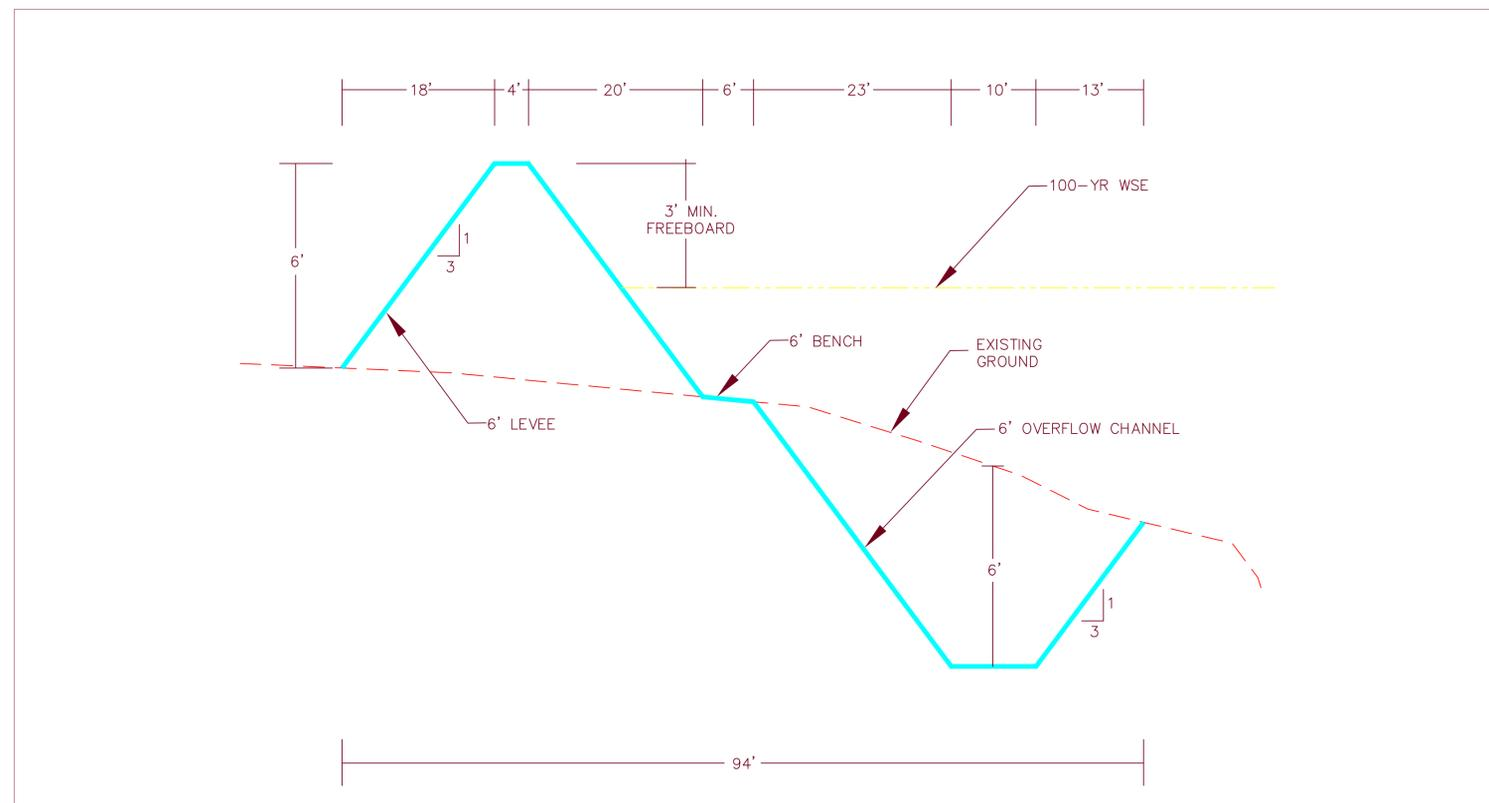
**LEVEE AND OVERFLOW CHANNEL DETAIL**
